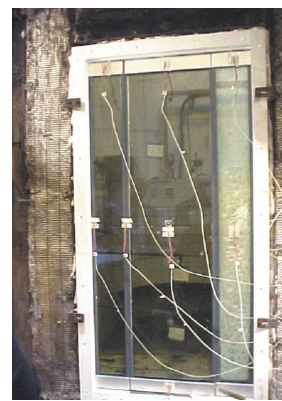
Fire glazing test
